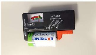
How to test the batteries: simply push the red slider as far to the right as it will go and insert the battery into the space (with positive charge on the right, next to the slider). Read the display to check that is says 'good'.
