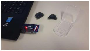
How to check the SD card: slot the SD card into the SD card reader (the writing on the SD card should be facing upwards) OR use the SD card port on your computer if you have one. Now insert the SD card reader into the USB port of your computer; a red light will show on the SD card reader when connected (Note: not all card readers may have a light). A dialogue
