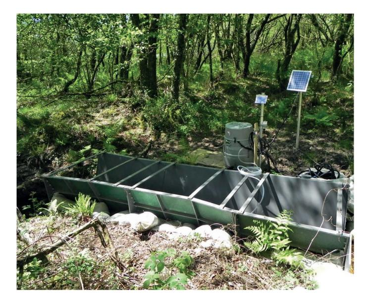
University of Exeter installed an instrumented flume at Stowford Moor to monitor run-off rates from a Culm grassland sub-catchment
