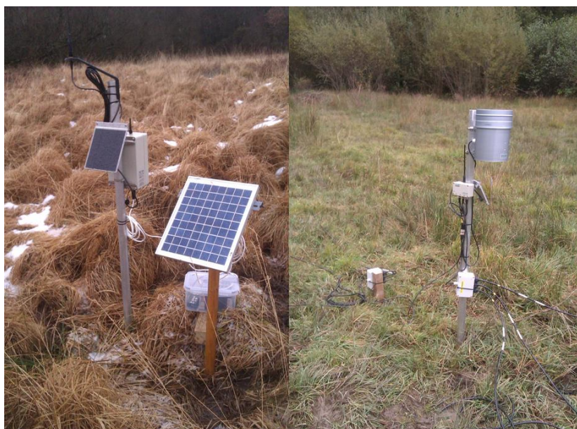
Figure 1.9. Left: RA440 telemetry base station at Stowford Moor, used to transmit data from field instrumentation on a 15 min time step over a 3G network. Right: Tipping bucket rain gauge at Halsdon; with junction boxes and cables leading to instrumented dipwells and an addIT radio unit to transmit data to the RA440 base station (© Alan Puttock).
